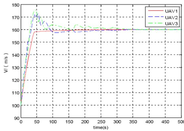
FIGURE 7. Velocity curves of three UAVs
