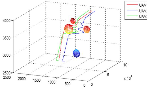
FIGURE 6. Flight trajectories of three UAVs in obstacles space
