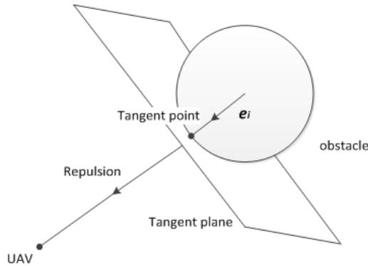
FIGURE 1. The repulsion schematic diagram of obstacle to UAV in 3D space
