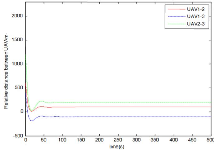
FIGURE 5. Relative distance curves between pairs of UAVs
