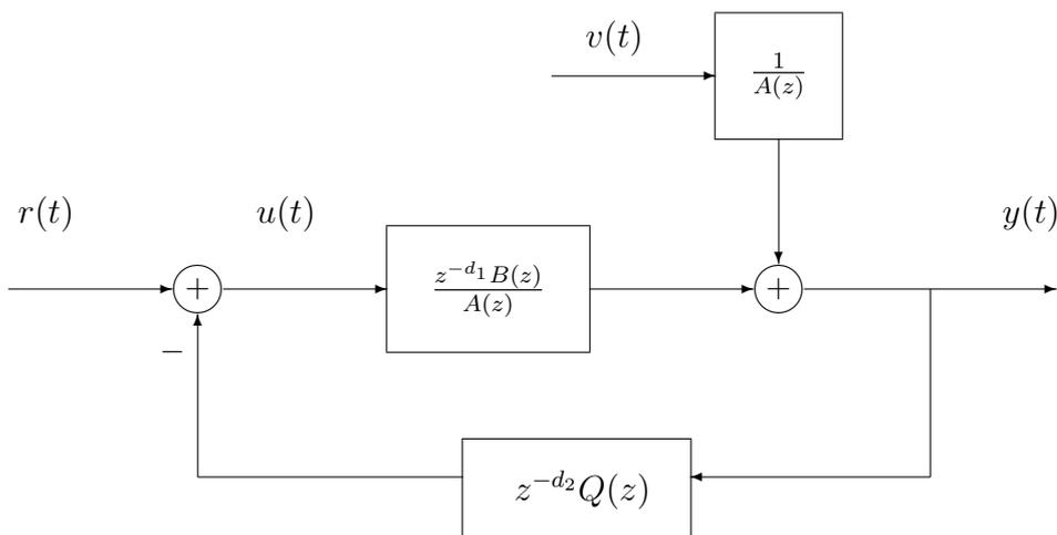
FIGURE 1. An SISO closed-loop system
