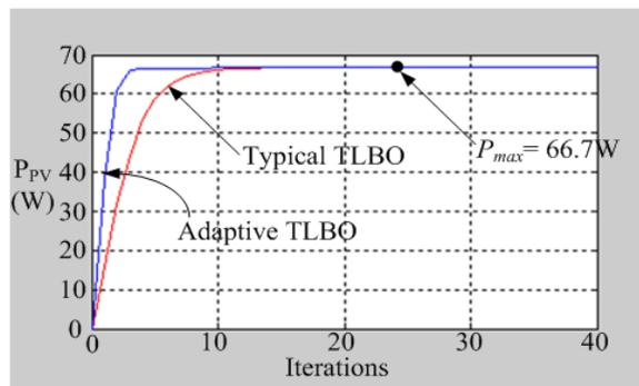
FIGURE 10. Tracking performance comparison between the presented adaptive TLBO algorithm and a typical counterpart in Case 4
