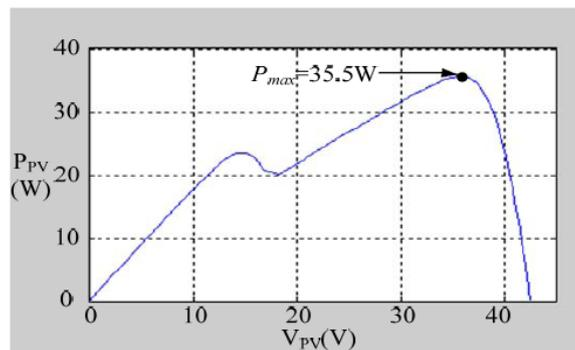
FIGURE 3. A simulated P-V characteristic curve for Case 1
