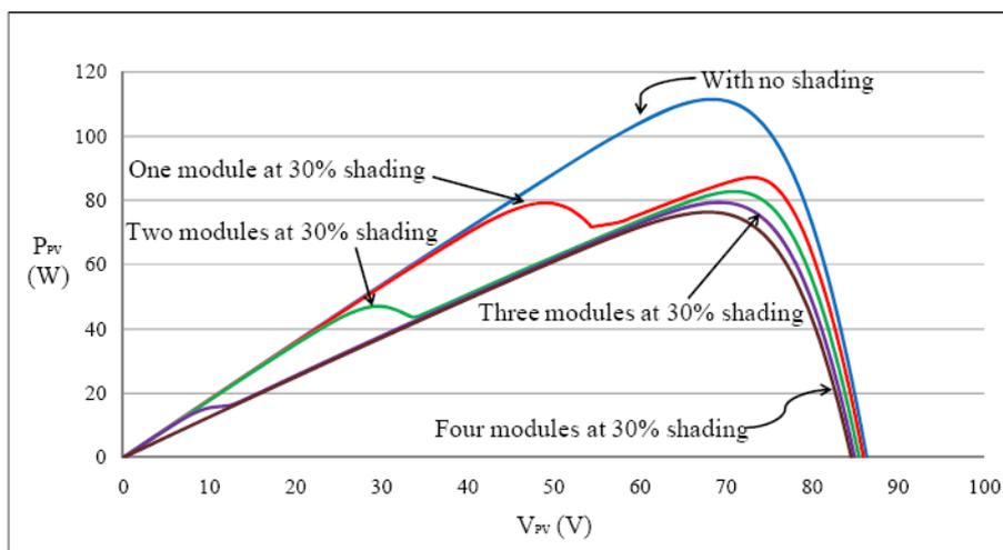
FIGURE 2. A family of P-V characteristic curves for a 4-series-1-parallel PVMA with the number of 30% shaded modules as a parameter
