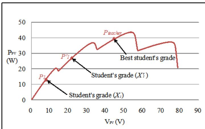
FIGURE 1. An illustration of the adaptive tracking mechanism via the tuning parameter  $T_F$
