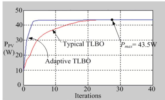
FIGURE 8. Tracking performance comparison between the presented adaptive TLBO algorithm and a typical counterpart in Case 3
