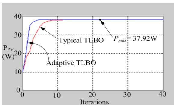
FIGURE 6. Tracking performance comparison between the presented adaptive TLBO algorithm and a typical counterpart in Case 2
