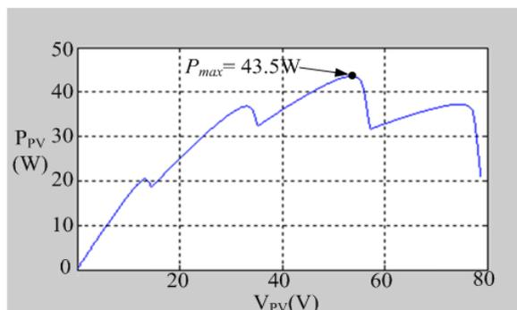
FIGURE 7. A simulated P-V characteristic curve for Case 3
