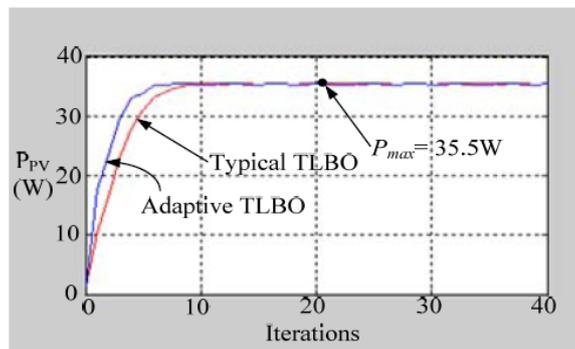
FIGURE 4. Tracking performance comparison between the presented adaptive TLBO algorithm and a typical counterpart in Case 1
