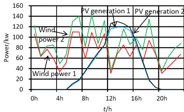
FIGURE 3. Typical daily power curves of each micro-grid's wind and PV generation
