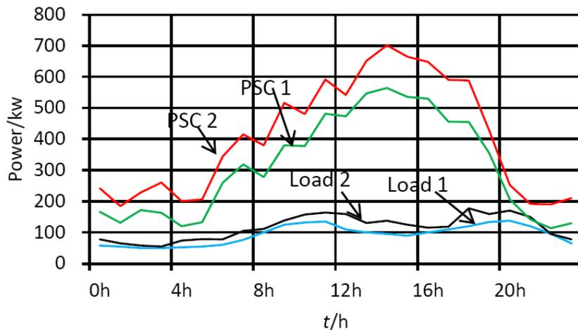
FIGURE 5. The curves of power supply capability of each micro-grid
