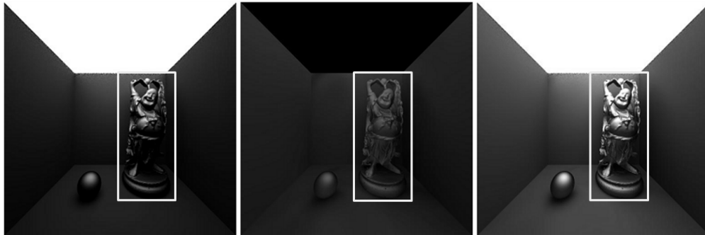
FIGURE 4. Rendering comparison and from left to right: direct illumination, indirect illumination and global illumination
