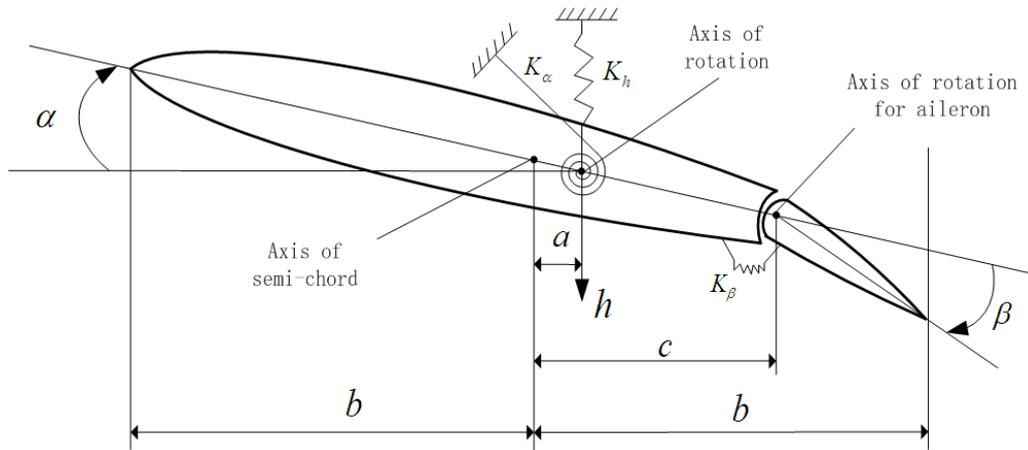
FIGURE 1. Airfoil section with control surface
