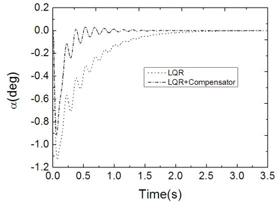
FIGURE 7. Time histories of pitch motion with controller and compensator
