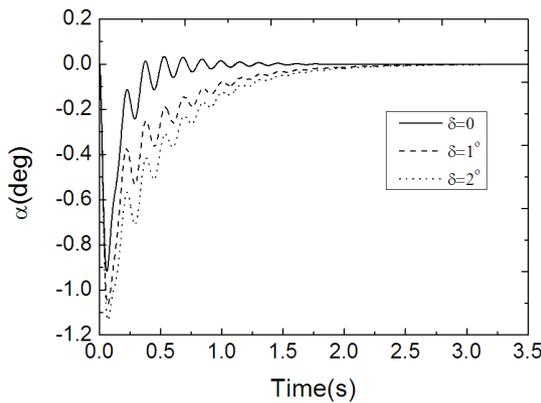
FIGURE 6. Time histories of pitch motion with controller
