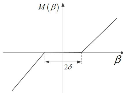
FIGURE 2. Control surface freeplay
