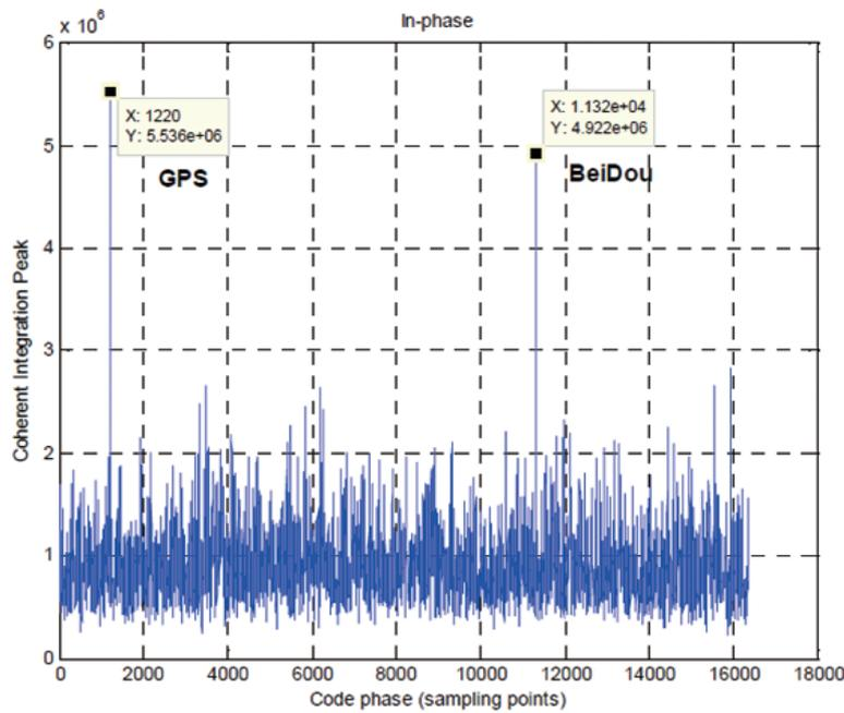
FIGURE 4. Combined GPS/BeiDou acquisition result using two visible satellites
