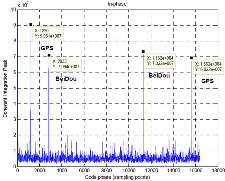
FIGURE 5. Combined GPS/BeiDou acquisition result using four visible satellites
