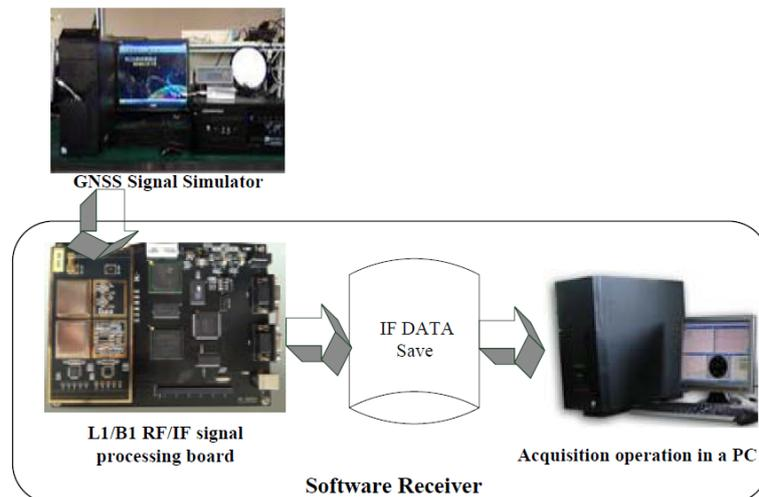
FIGURE 2. Simulation platform
