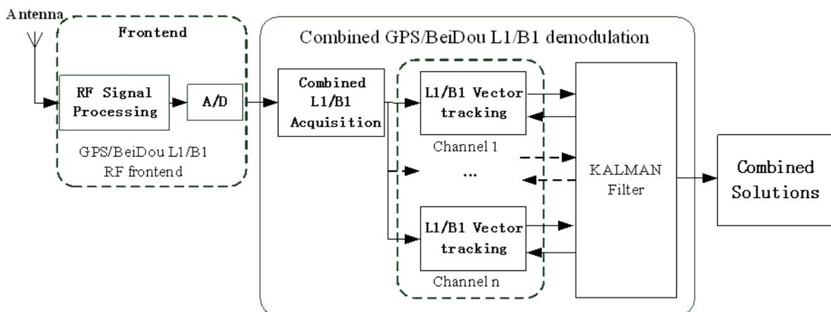
FIGURE 1. Combined GPS/BeiDou L1/B1 receiver architecture
