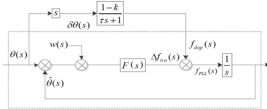
FIGURE 2. Aided tracking loop  $s$ -domain schematics
