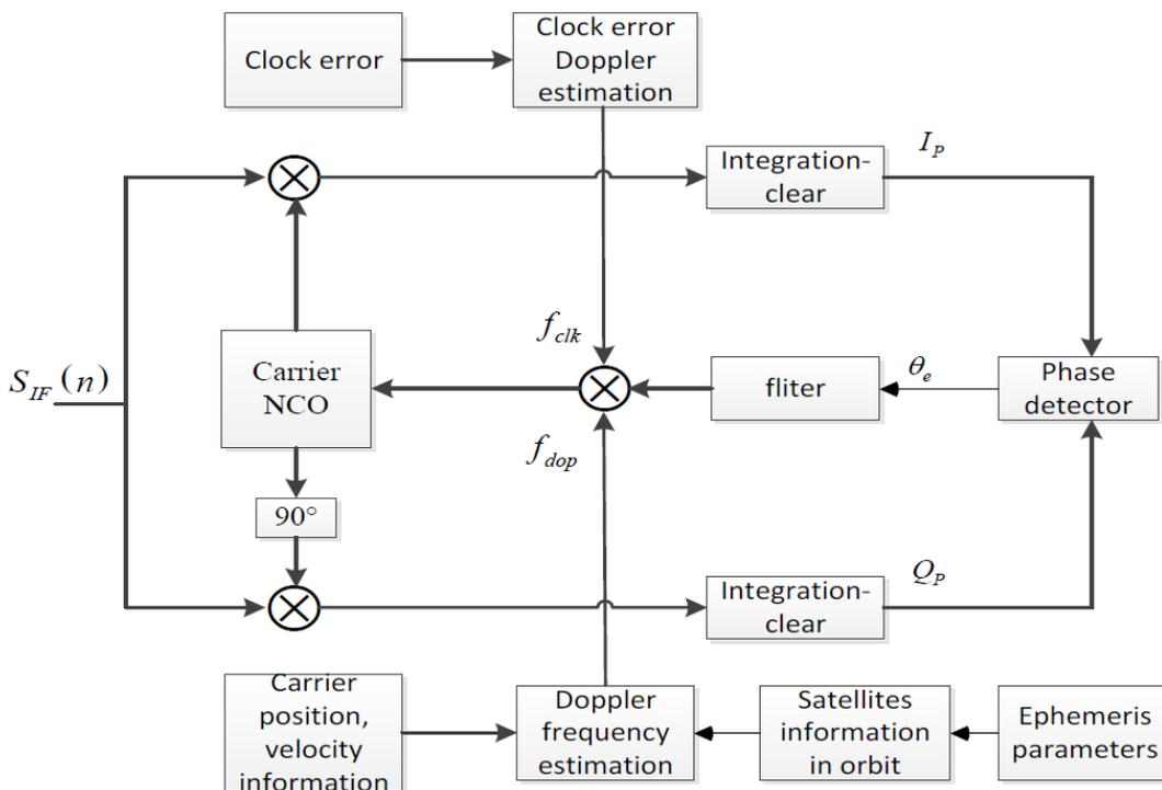
FIGURE 1. INS-aided receiver carrier tracking loop design
