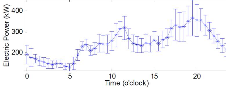
FIGURE 3. The change of average electric power
