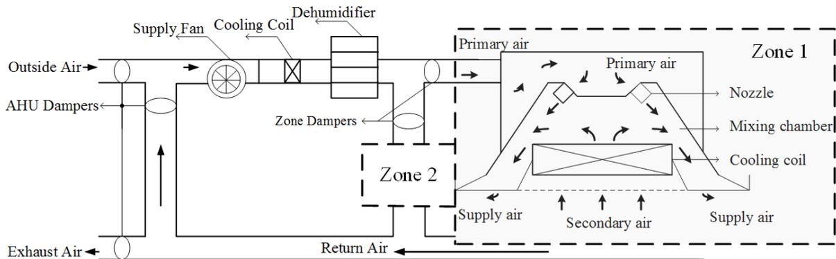
FIGURE 1. Schematic diagram of HVAC system with ACB terminals
