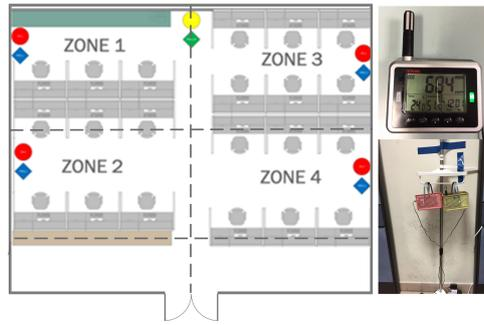
FIGURE 2. Test site and sensor layout of multiple zones
