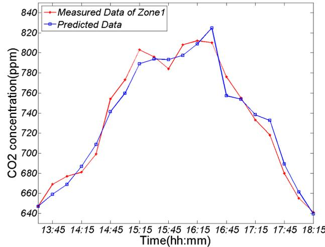
FIGURE 7. Prediction of  $CO_2$  concentration by using the identified parameters
