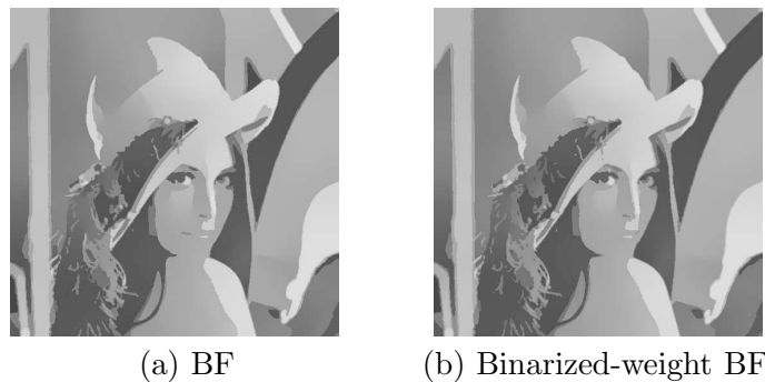
FIGURE 3. Images using the BF ( T_1 = 20 ) and binarized-weight BF ( T_1 = 12 , C = 3.0 )
