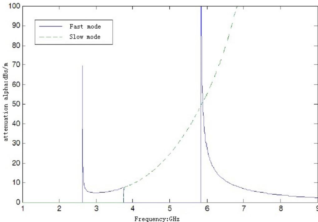
FIGURE 4. The theoretical attenuation constants (series resistance  $r = 0.01125\Omega\cdot\text{m}$ )
