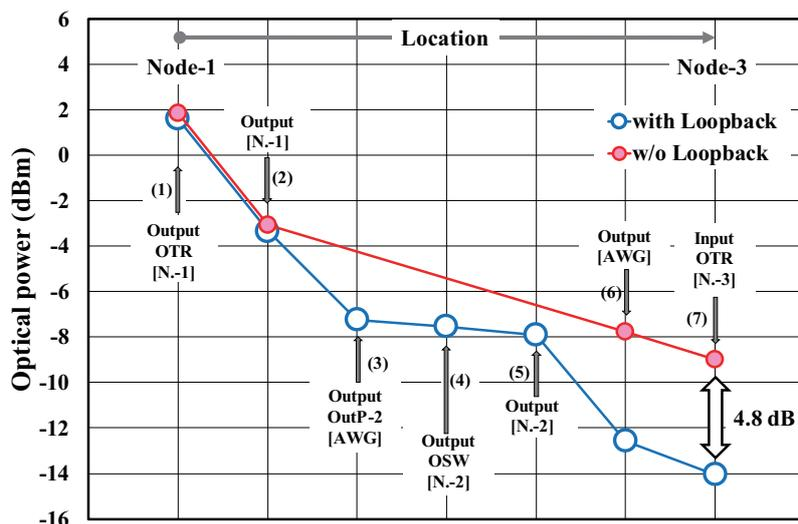
FIGURE 8. Measured optical powers corresponding to looped-back wavelength path ( $\lambda_2$ ) and direct wavelength path ( $\lambda_3$ )
