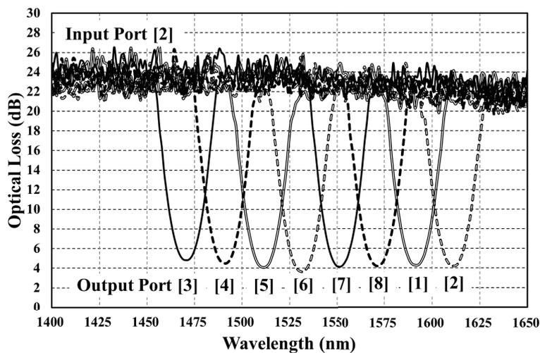
FIGURE 4. AWG optical losses from input port [2] to other ports
