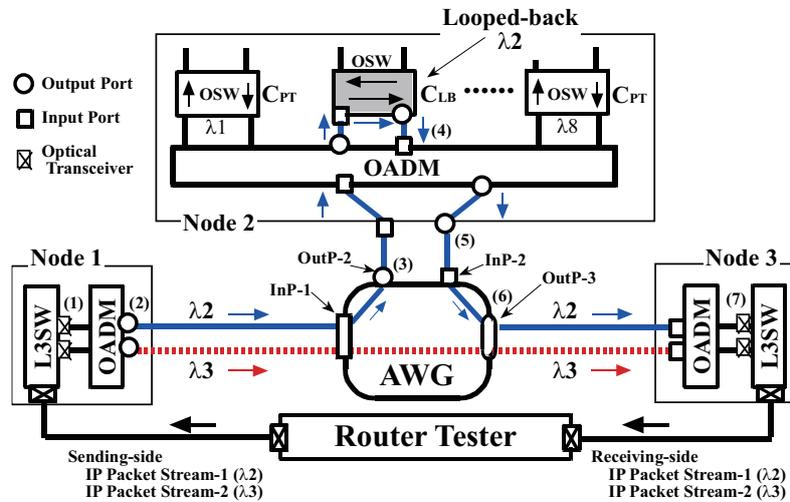
FIGURE 5. Experimental network and setting for evaluating wavelength path relocation performance
