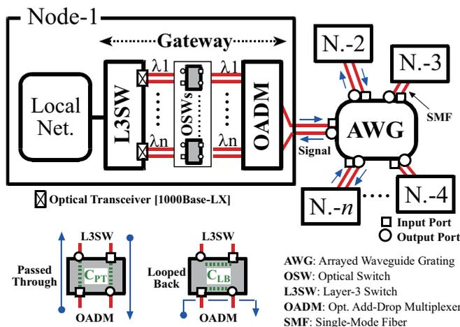
FIGURE 1. Schematic of AWG-STAR network with wavelength path relocation function
