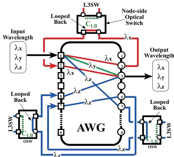
FIGURE 2. Loopback by switching OSWs
