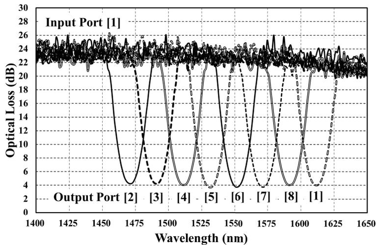
FIGURE 3. AWG optical losses from input port [1] to other ports
