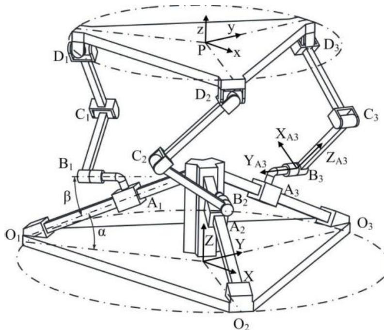
FIGURE 1. The sketch of 3-PRRU parallel mechanism
