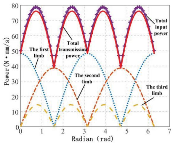
FIGURE 6. Comparison between input power and transmission power of limb with parameter  $\beta = 15^\circ$
