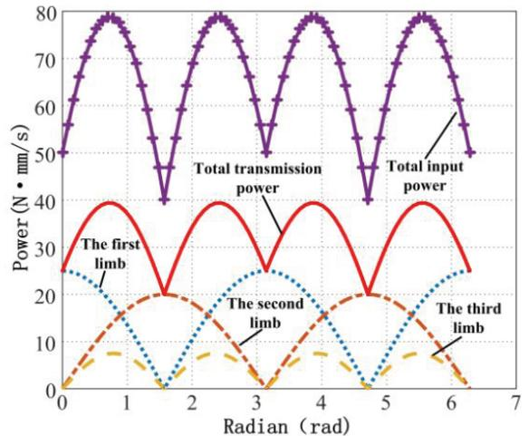
FIGURE 8. Comparison between input power and transmission power of limb with parameter  $\beta = 60^\circ$
