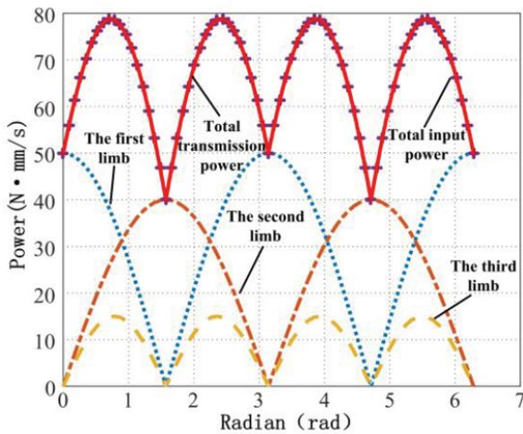
FIGURE 5. Comparison between input power and transmission power of limb with parameter  $\beta = 0^\circ$
