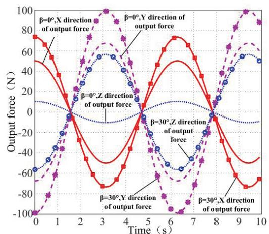
FIGURE 10. Output force curve of moving platform
