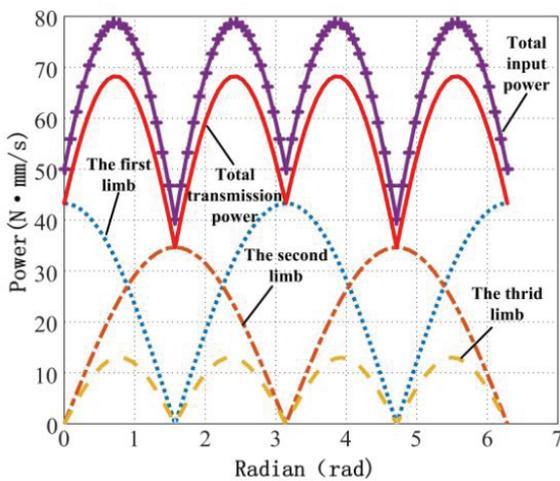
FIGURE 7. Comparison between input power and transmission power of limb with parameter  $\beta = 30^\circ$
