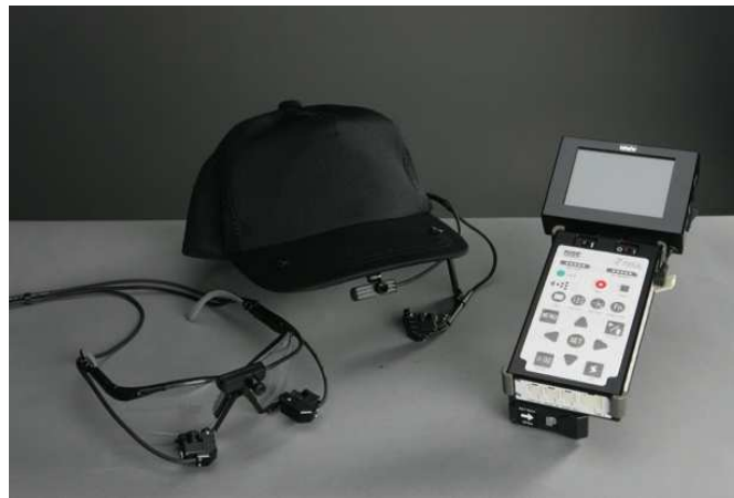
FIGURE 3. Eye-mark recorder (EMR-9)
