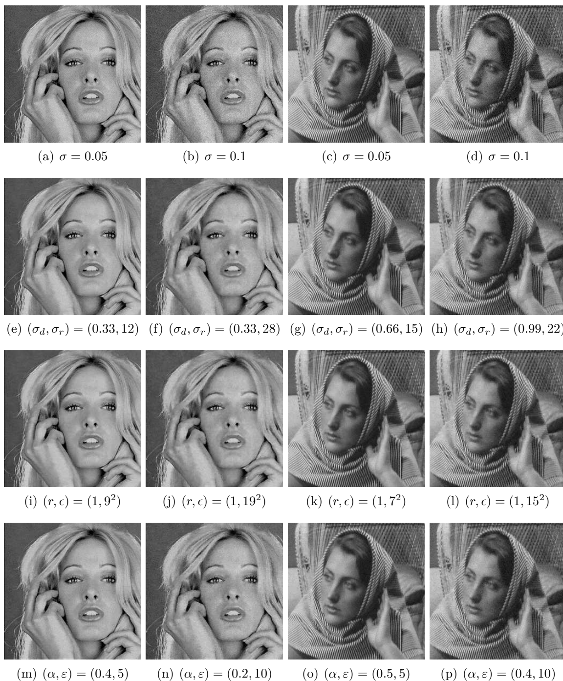
FIGURE 4. Filtering result for “Woman” and “Barbara” corrupted by Gaussian noise. (a)-(d) Noise-corrupted input images, (e)-(h) filtering results by the bilateral filter, (i)-(l) filtering results by guided filter, (m)-(p) filtering results by the proposed method.
