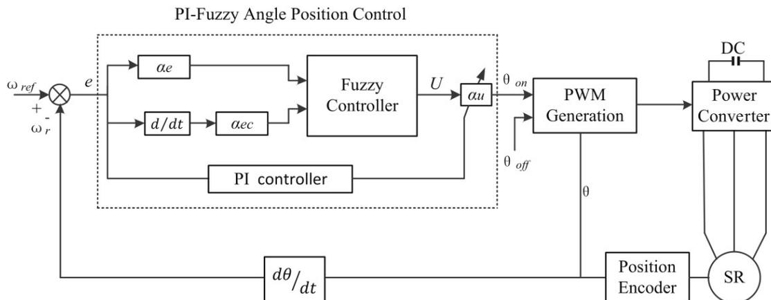
FIGURE 4. Control system of SRM
