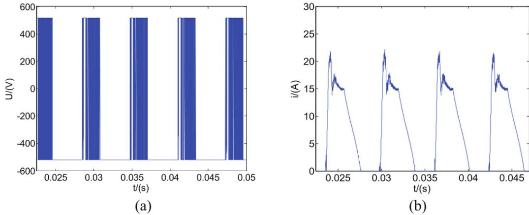
FIGURE 5. Performance of SRM: (a) a phase voltage and (b) a phase current
