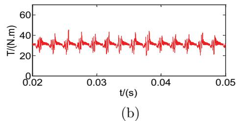
FIGURE 8. The comparison of torque: (a) PI-fuzzy algorithm and (b) fuzzy algorithm
