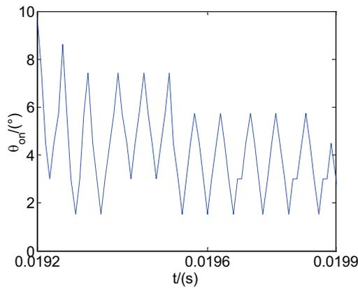
FIGURE 6. Turn-on angle of SRM
