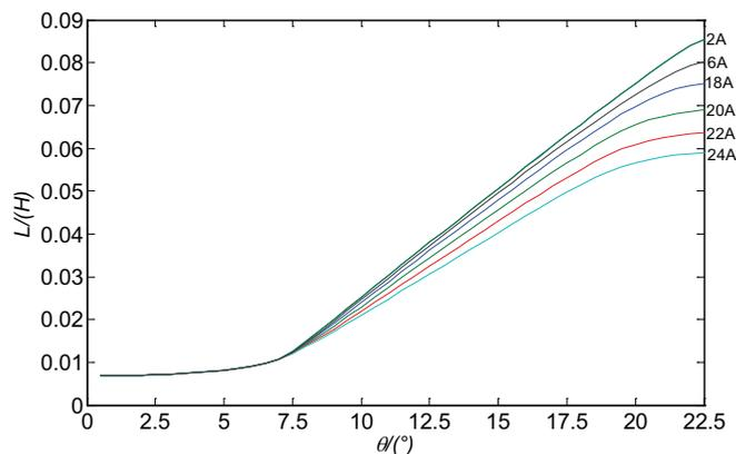
FIGURE 1. Inductance characteristics for the SRM
