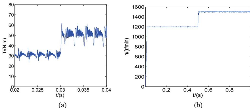
FIGURE 9. Dynamic characteristic of SRM: (a) torque and (b) speed
