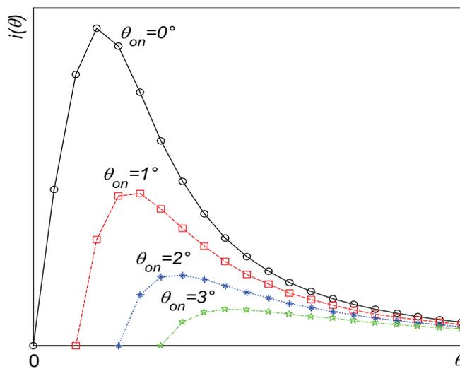
FIGURE 3. Current in different turn-on angles
