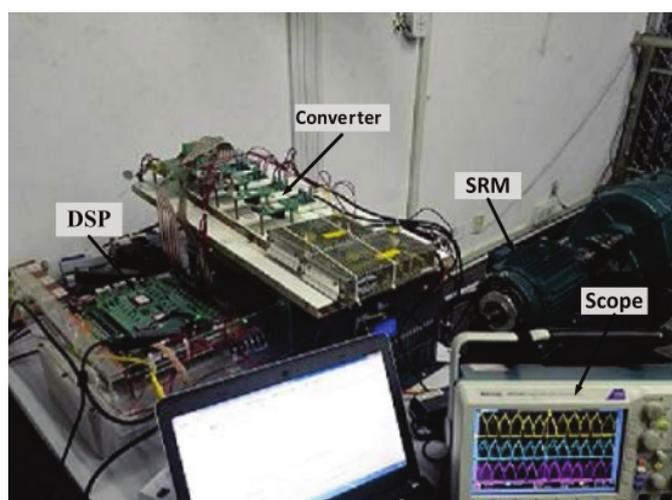
FIGURE 10. Hardware platform of system
