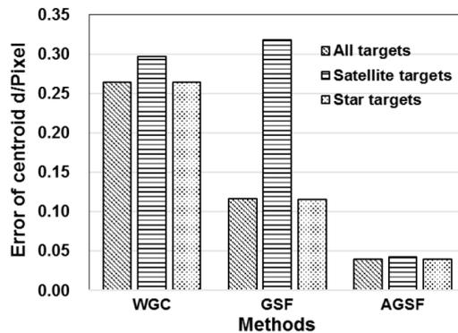
FIGURE 6. Real data test: from left to right the average error of all targets, the satellite targets and the star targets of each method
