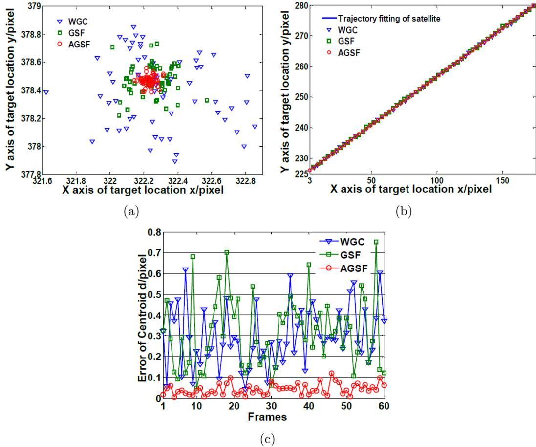
FIGURE 5. Results of real data: (a) center extraction results from different methods for one star, (b) the positioning results for one satellite and the trajectory fitting result, (c) centroid errors of each method for the satellite
