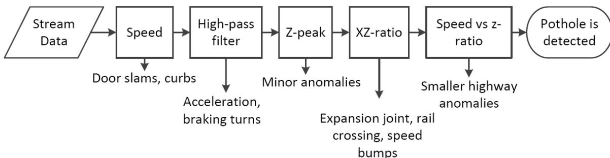
FIGURE 1. The flowchart of the pothole detection procedure [9]
