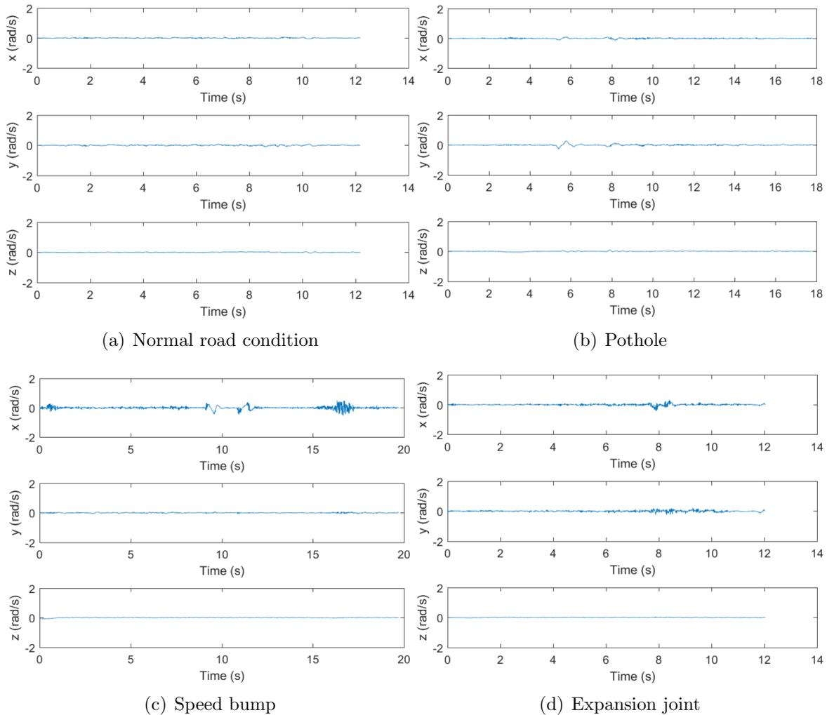
FIGURE 4. The typical recorded vehicle rates of rotations in  $x$ -,  $y$ -, and  $z$ -directions when the the probe vehicle runs over a normal road condition, a road with a pothole, a road with a speed bump, and a road with an expansion joint. Those directions are related to the vehicle pitch, roll, and yaw, respectively.
