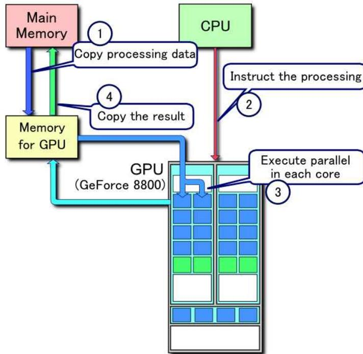
FIGURE 2. Processing flow on CUDA
