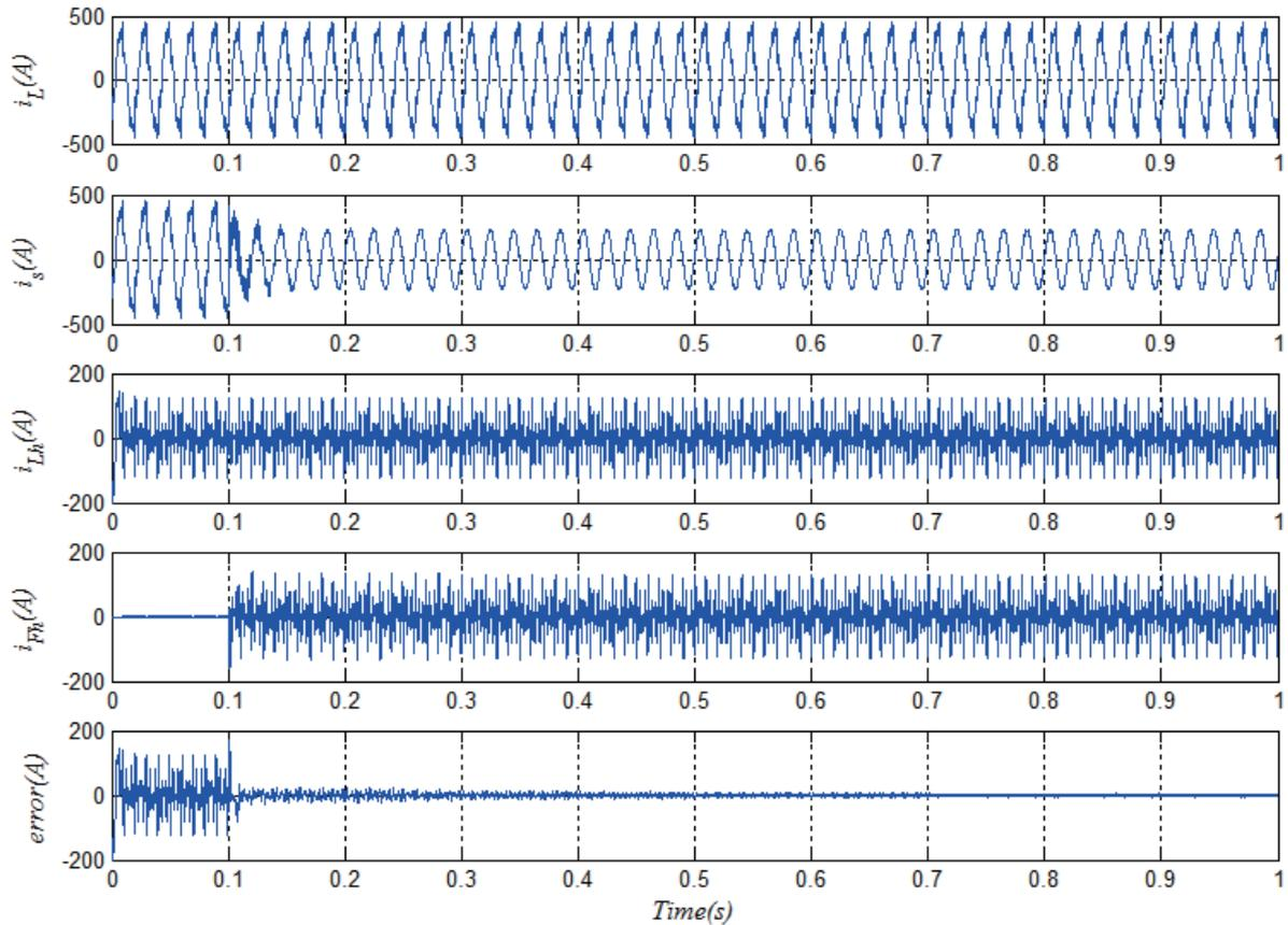
FIGURE 4. Dynamic response of HAPF with the Generalized PI controller
