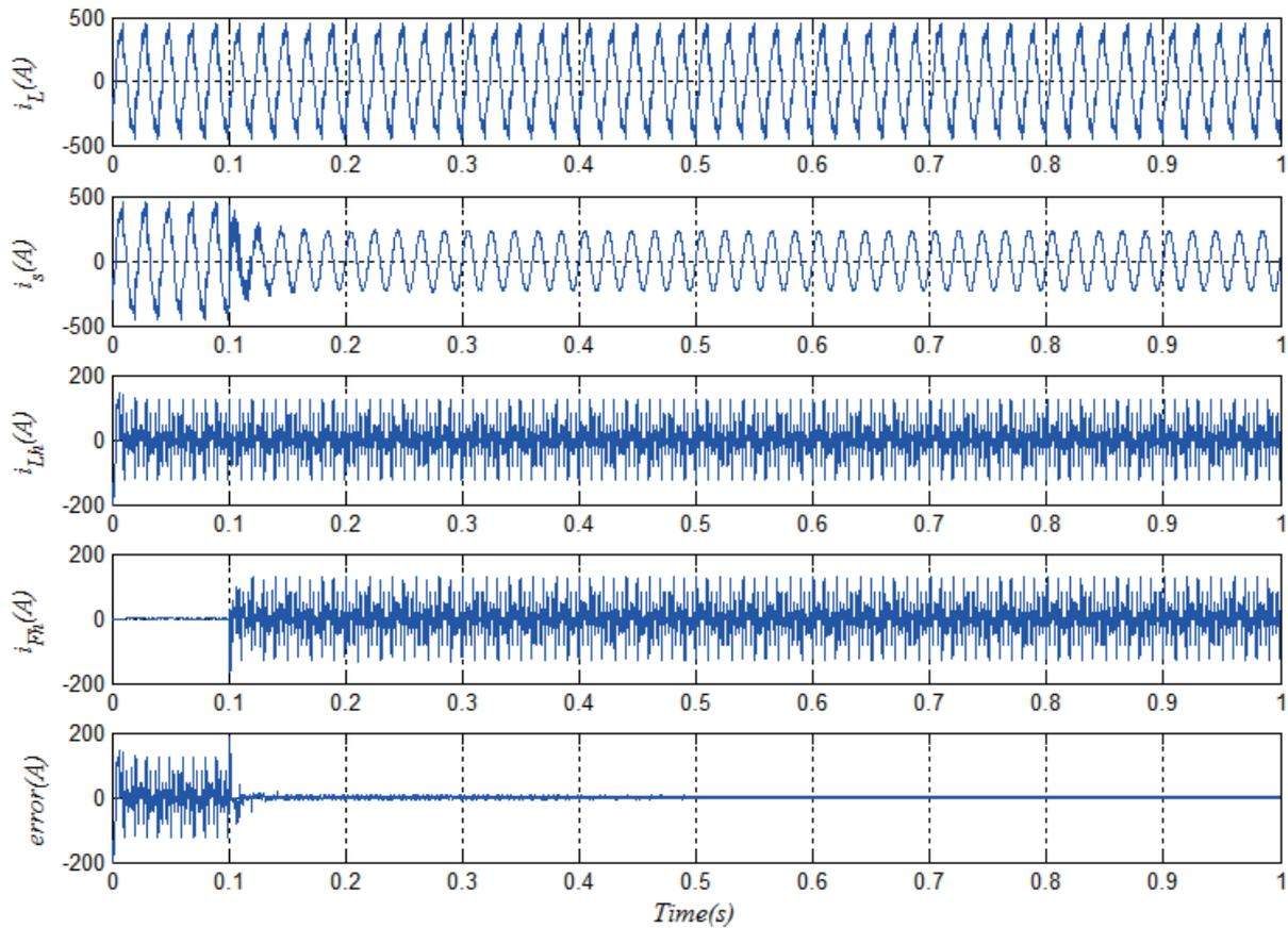
FIGURE 5. Dynamic response of HAPF with the proposed controller
