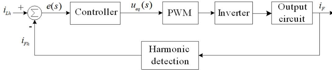
FIGURE 2. Control block diagram for HAPF
