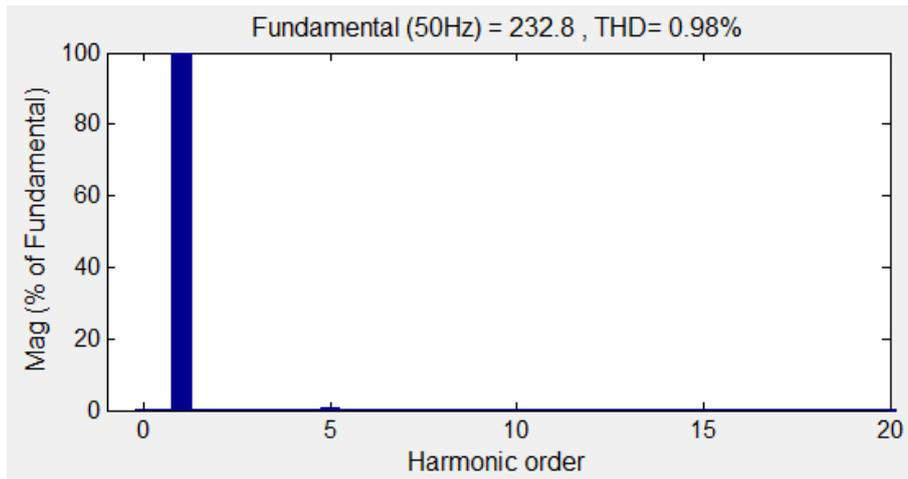
FIGURE 6. THD of  $i_s$  in steady-state with the Generalized PI controller
