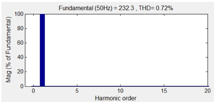
FIGURE 7. THD of  $i_s$  in steady-state with the proposed controller
