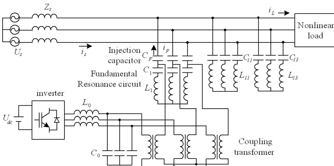
FIGURE 1. Topology of the Hybrid Active Power Filter
