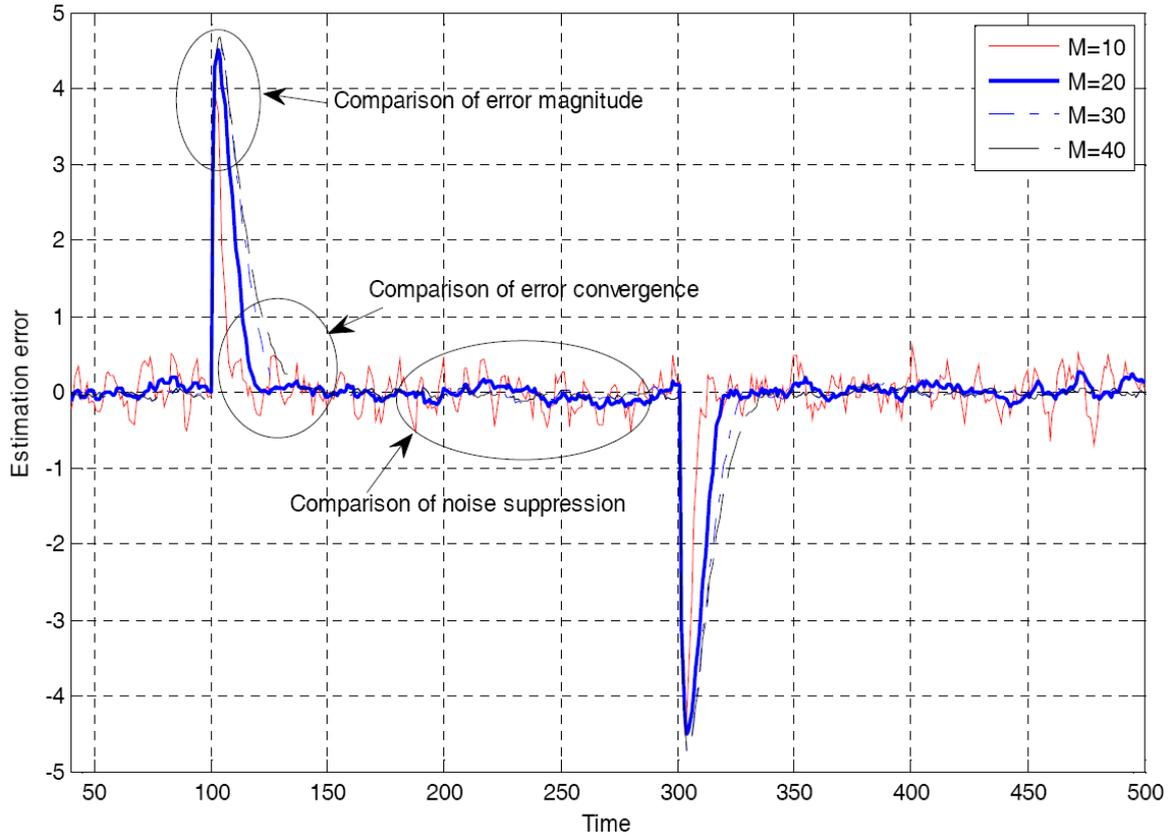
FIGURE 3. Simulation results for unknown input according to diverse window lengths
