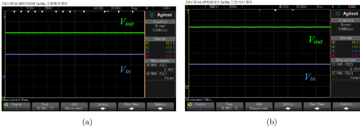
FIGURE 6. Input voltage and output voltage of the traditional converter when the output capacitor is 22 \mu\text{F} . (a) R_L = 2.2 \text{ M}\Omega and (b) R_L = 470 \text{ k}\Omega .
