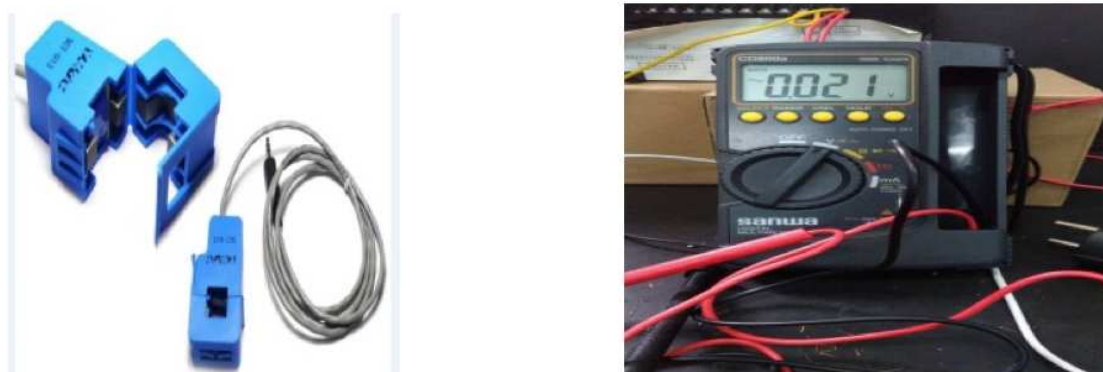
FIGURE 5. Current sensor of SCT013 and calibration tool
