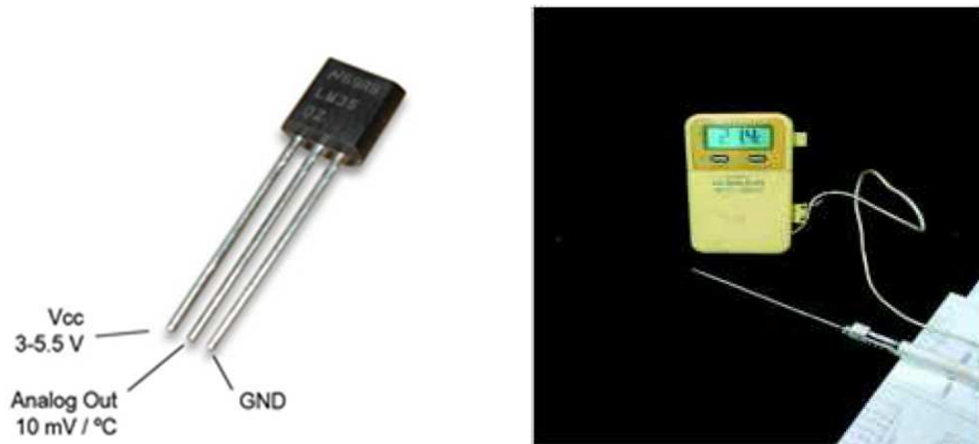
FIGURE 6. Temperature sensor of LM35 and calibration tool
