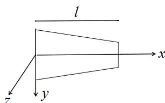
FIGURE 1. Variable section cantilever beam diagram
