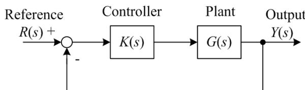
FIGURE 1. General structure of control system
