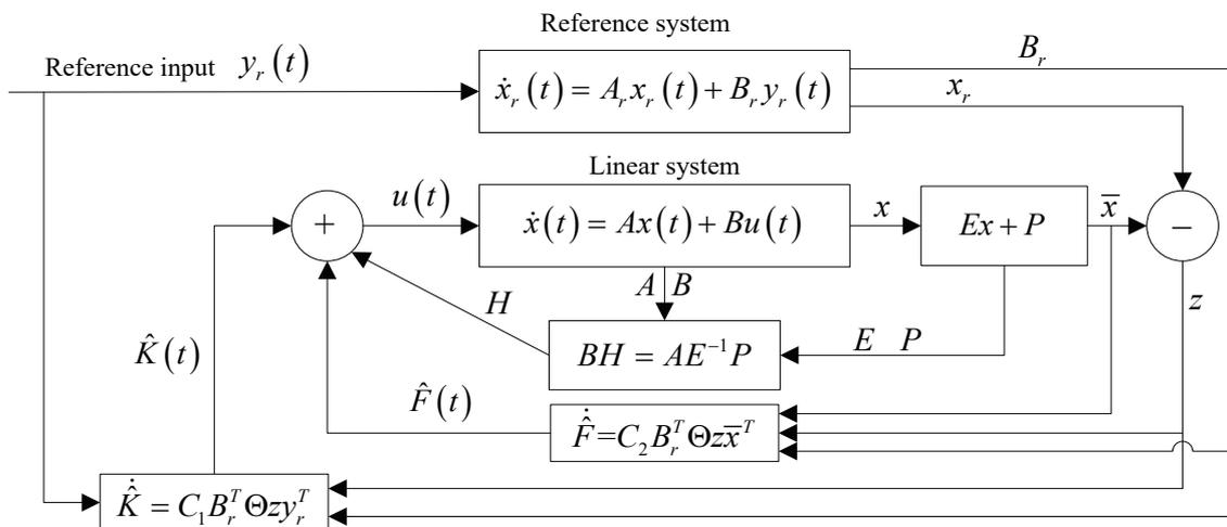
FIGURE 1. Diagram of model reference shape asymptotic tracking control
