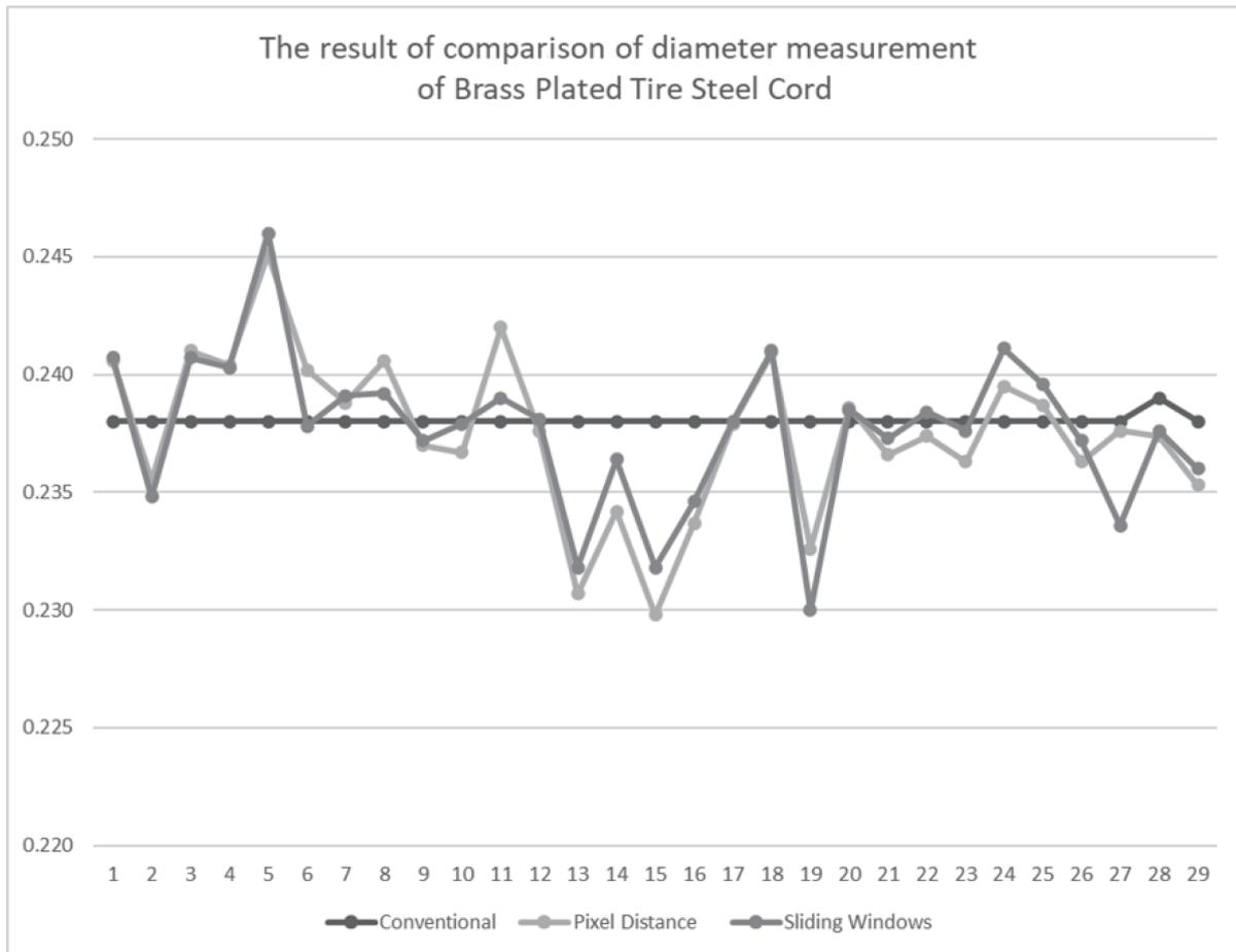
FIGURE 7. The results of comparison of diameter measurements of brass plated tire steel cord
