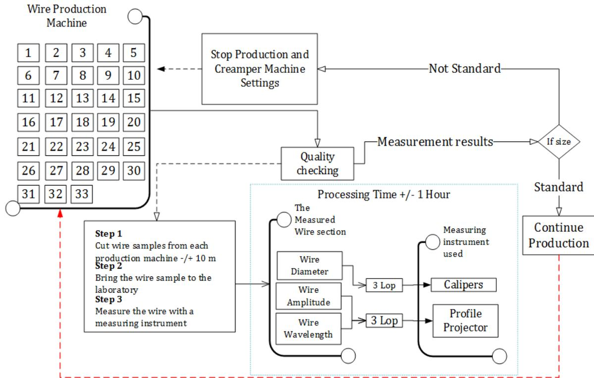
FIGURE 3. Simulation of brass plated tire steel cord production
