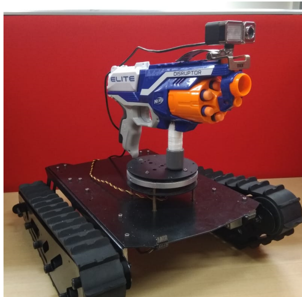
FIGURE 1. Prototype of a tank-based military robot using computer vision
