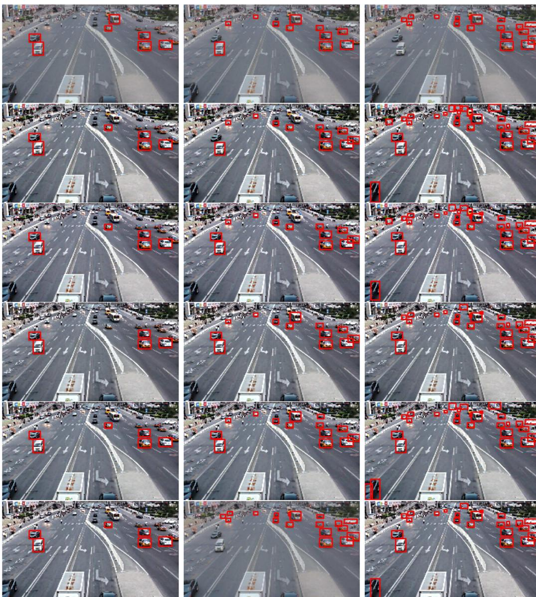
FIGURE 3. Qualitative comparison of various object detectors with detail manipulation on low quality MV\_40711 dataset. First column: NAS; Second column: GA; Third column: FA. First row: None; Second row: GF; Third row: DGF; Fourth row: DGFA; Fifth row: DCGF; Sixth row: DCGFA.
