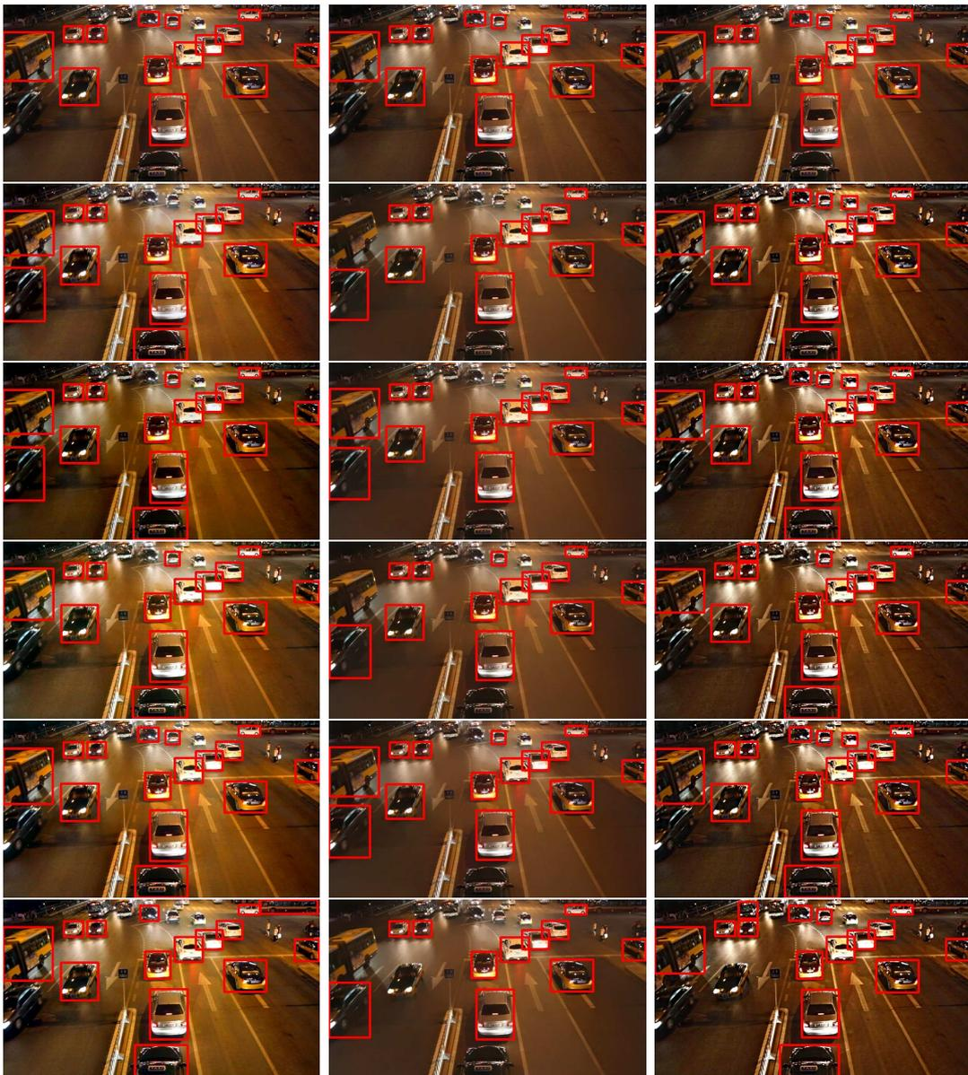
FIGURE 2. Qualitative comparison of GA object detector with edge-aware filtering applications on MV\_40755 dataset. First column: Tonal adjustment; Second column:  $L_0$  smoothing; Third column: Detail manipulation. First row: None; Second row: GF; Third row: DGF; Fourth row: DGFA; Fifth row: DCGF; Sixth row: DCGFA.
