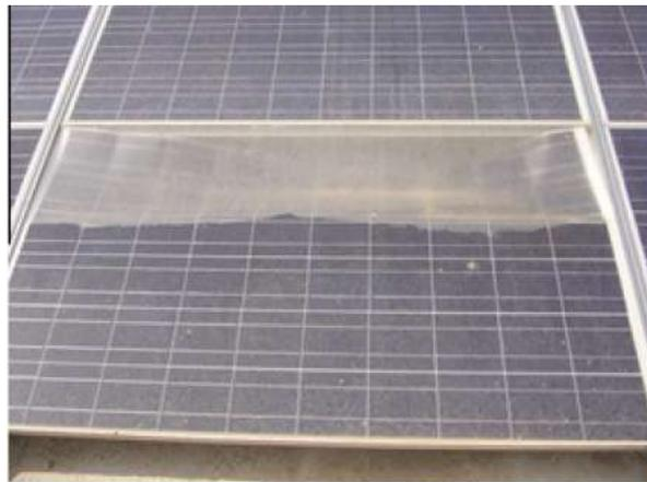
FIGURE 2. A PV module with delamination [10]
