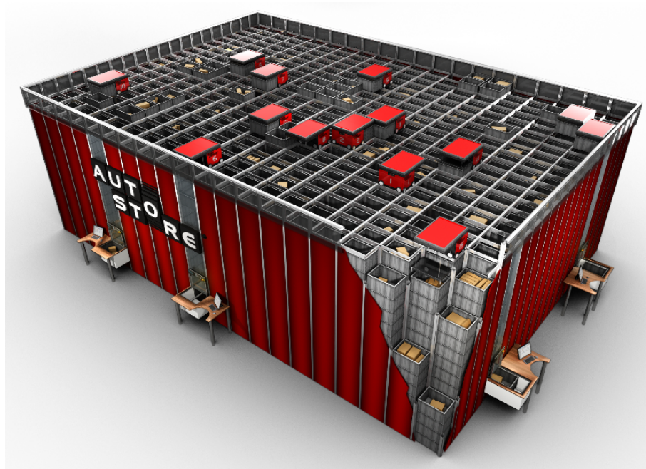
FIGURE 1. Schematic view of the AutoStore™ system (image source: itersnews.com)
