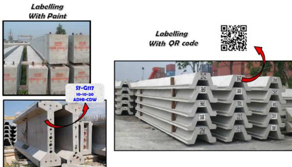
FIGURE 3. Types of labels on current precast concrete products
