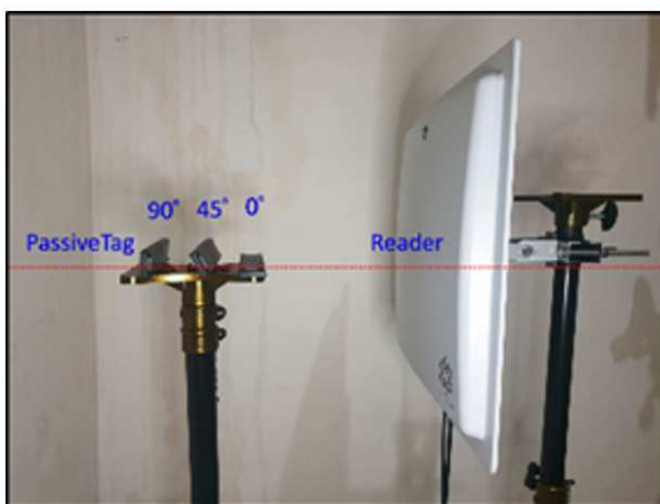
FIGURE 8. Orientation of tag position
