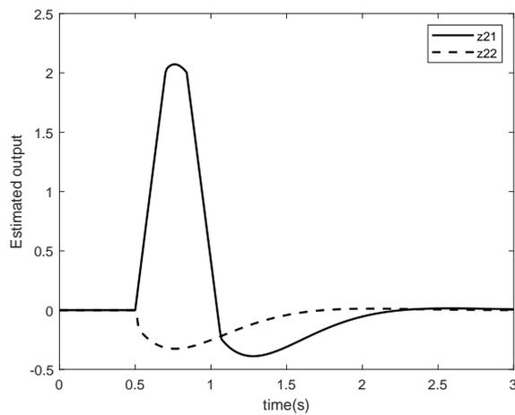
FIGURE 4. Estimation of disturbances via LESO
