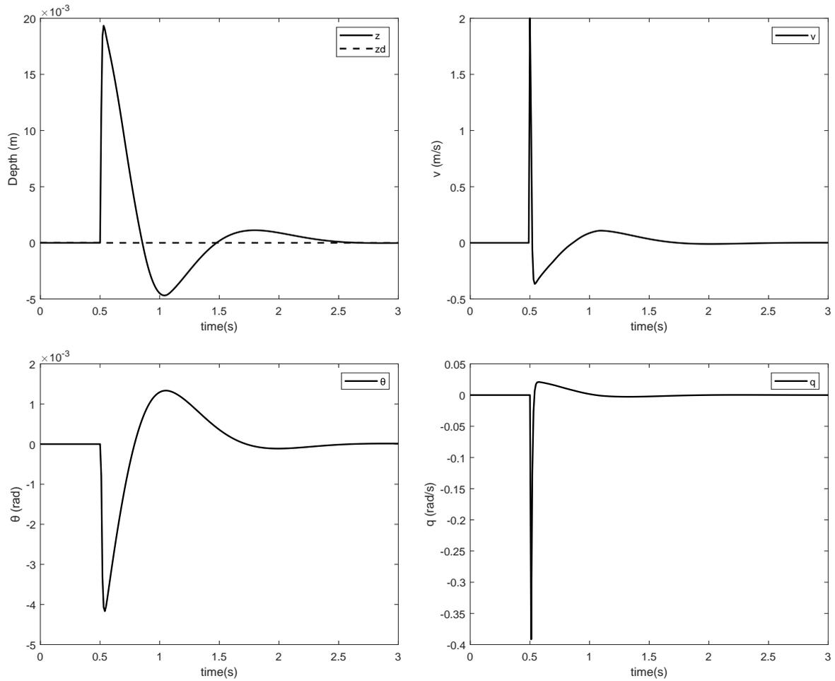
FIGURE 3. Tracking responses with external disturbance
