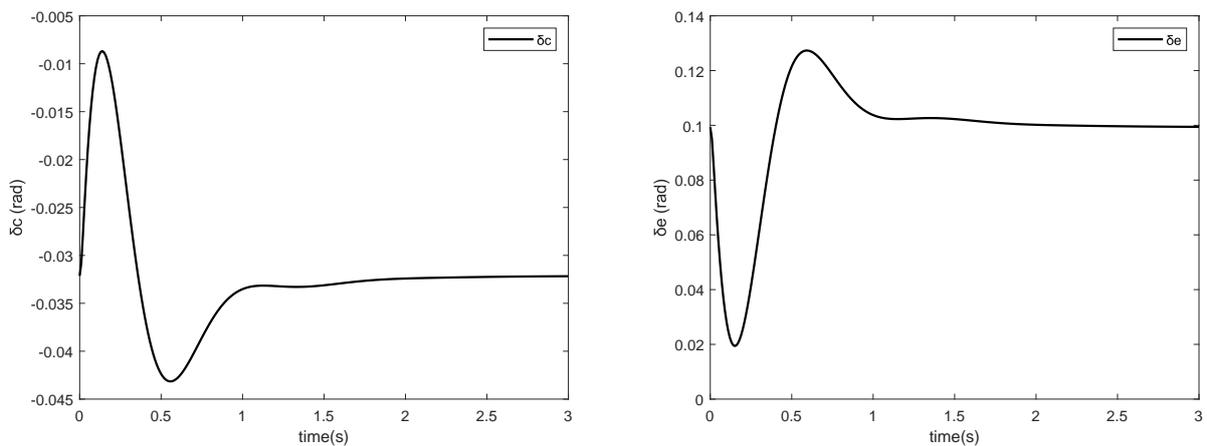
FIGURE 2. Control actions due to depth step input
