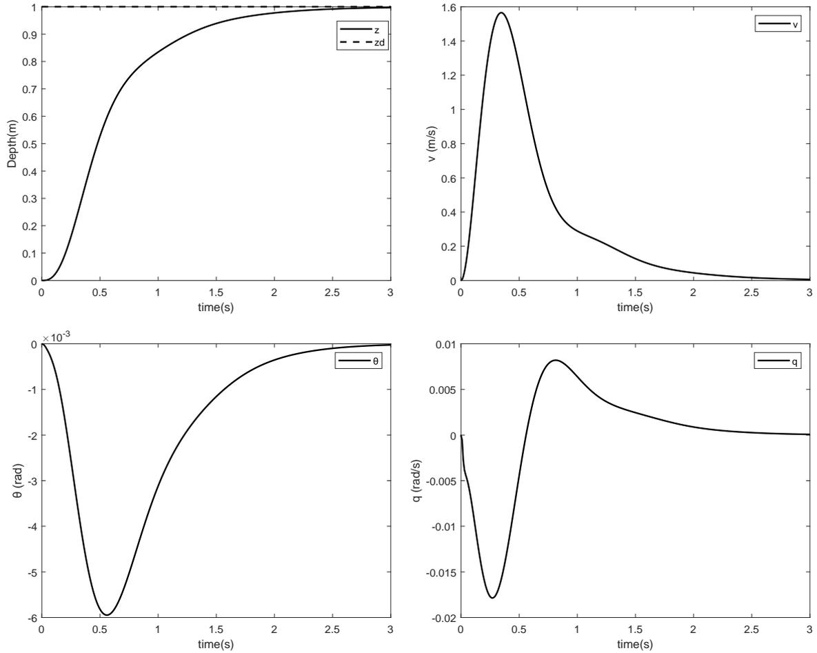
FIGURE 1. Tracking responses due to depth step input
