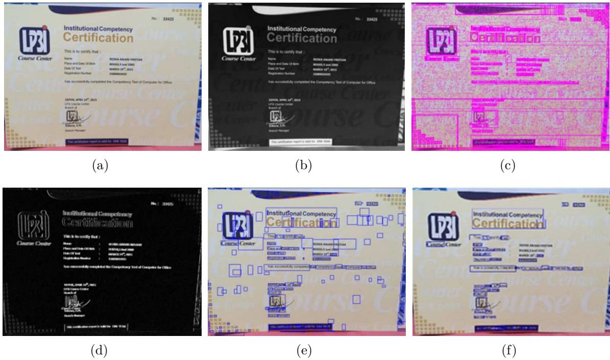
FIGURE 2. Examples of detection results: (a) Initial image, (b) negative grayscale image, (c) the Maximum Tree result, (d) the vertical Sobel, (e) text candidates, and (f) final bonding box
