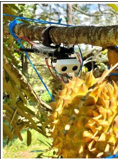
FIGURE 9. Device IoT durian fall detector on set (Zoom In)
