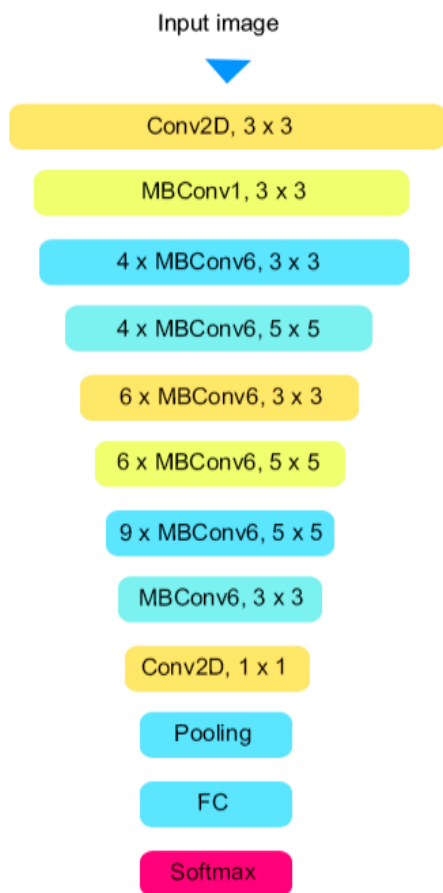
FIGURE 1. Architecture of EfficientNetB6
