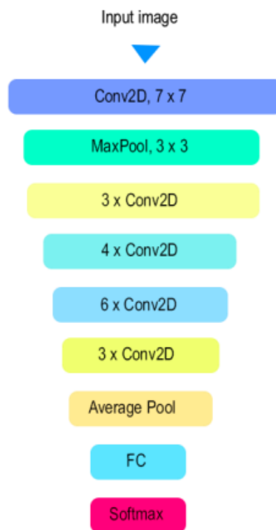
FIGURE 4. Architecture of ResNet50
