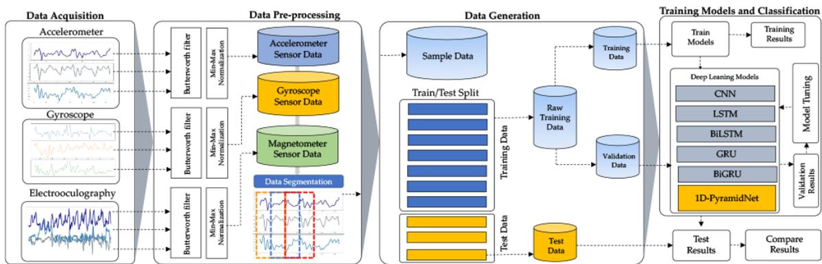
FIGURE 1. RST classification framework based on inertial sensors used in this work
