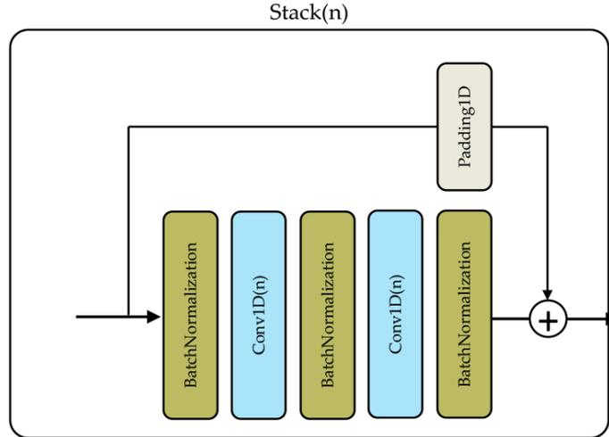
FIGURE 3. Structure of a stack block used in the proposed RST-PyramidNet
