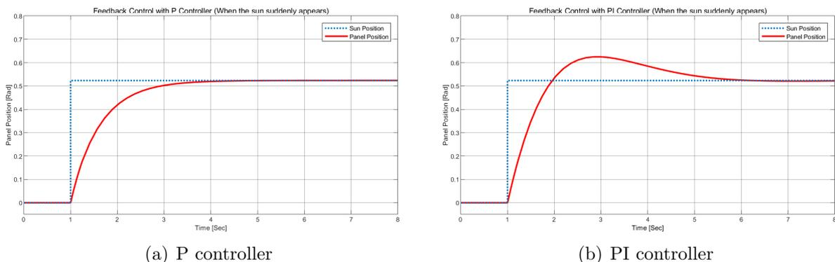
FIGURE 3. Feedback control with PID controllers when the sun suddenly appears
