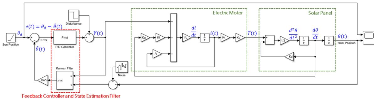
FIGURE 8. Overall block diagram for solar tracker
