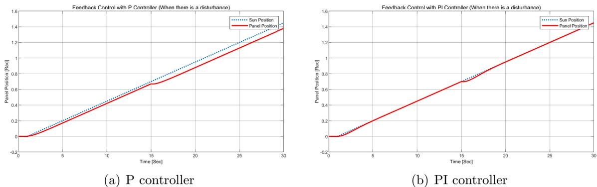
FIGURE 5. Feedback control with PID controllers when there is a disturbance
