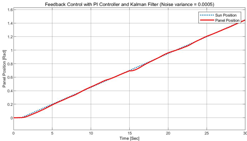
FIGURE 7. Feedback control with PI controller and Kalman filter
