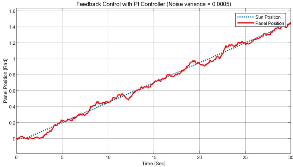
FIGURE 6. Feedback control with PI controller when there is a noise
