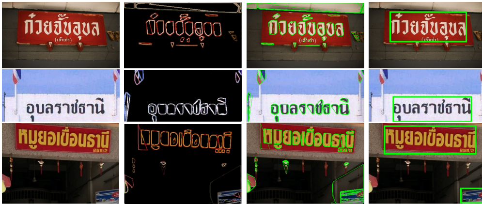
FIGURE 2. Example of the detection results: Column 1 displays the input images, Column 2 presents the MSER in the images, Column 3 shows the detected candidate texts, and Column 4 presents the identified text regions
